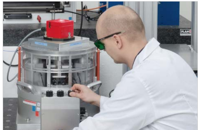
Geophone calibration on an SE-13 in the SPEKTRA laboratory
