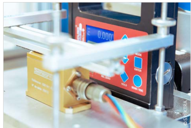
Example of an accredited calibration for an inclinometer.
