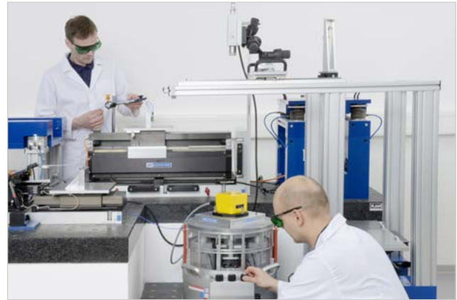
Primary calibration of a geophone in the SPEKTRA laboratory
