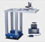
all-digital laser vibrometer incl. vibration isolation and positioning device for the laser head
